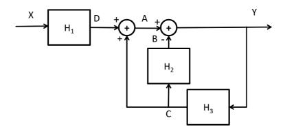
For simplicity we have omitted all the terms  $(e^{j\omega})$  in the diagram above. Unless otherwise stated uppercase letters will denote Fourier-domain variables and lower-case letters time-domain ones. We can now write all the system equations in Fourier domain:
