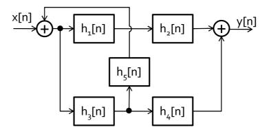
Express the frequency response of the overall system  $H(e^{j\omega})$  in terms of the frequency responses of the subsystems depicted in the diagram.
