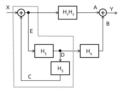
We can observe that there is a feedback loop involving the first addition operator and systems  $H_3$  and  $H_5$  (surrounded by a dashed line in the diagram above). The best way to proceed is to first compute the frequency response of the sub-system bounded by the dashed line, i.e. to find the relationship between D and X. We can see that the feedback sub-system contains 4 unknowns (X, E, D, C) which means that we will need to write 3 equations:
