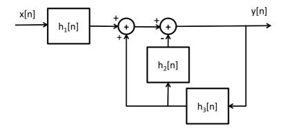
Express the frequency response of the overall system  $H(e^{j\omega})$  in terms of the frequency responses of the subsystems  $H_1(e^{j\omega})$ ,  $H_2(e^{j\omega})$ , and  $H_3(e^{j\omega})$ .
