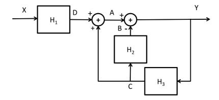
For simplicity we have omitted all the terms  $(e^{j\omega})$  in the diagram above. Unless otherwise stated uppercase letters will denote Fourier-domain variables and lower-case letters time-domain ones. We can now write all the system equations in Fourier domain:
