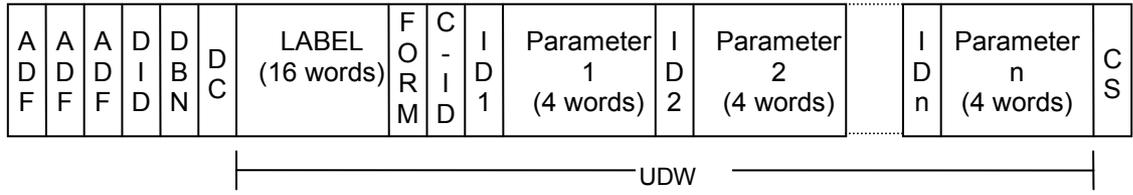
**Figure 6 — Binary-type camera positioning data packets (SMPTE 315M)**
