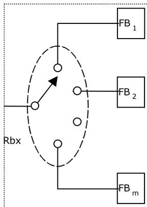
FB<sub>n</sub> is the M4Mux buffer for the elementary stream in M4Mux channel n
