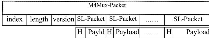
Figure 12 — Structure of M4Mux packet in MuxCode mode
