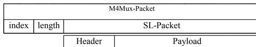
Figure 11 — Structure of M4Mux packet in simple mode
