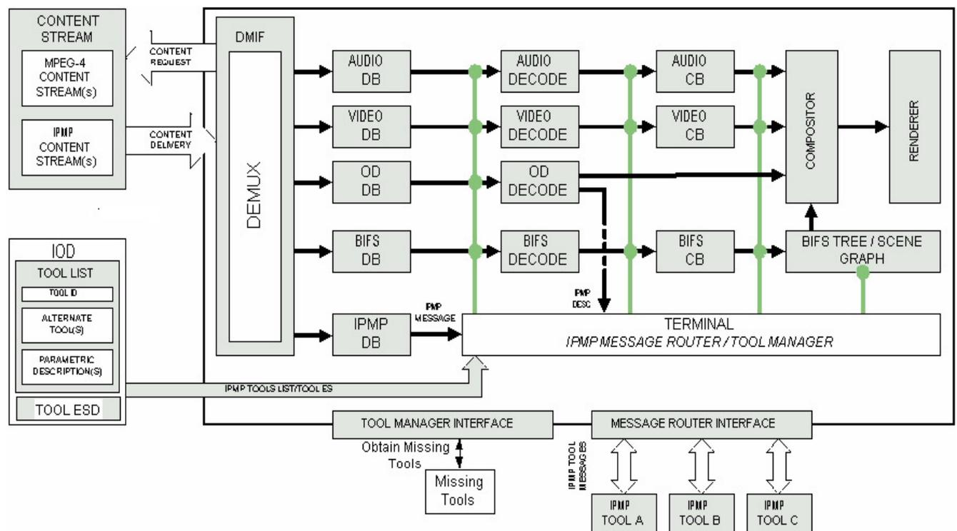
Figure 9 — IPMP system in the ISO/IEC 14496 terminal architecture
