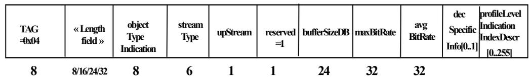
When present, the decSpecificInfo descriptor is an opaque descriptor (tag=0x05), configured according to the ObjectDescriptorID and to the streamType.
