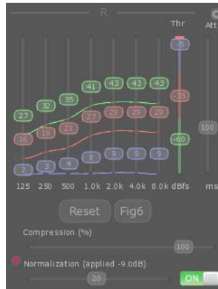
Figure 33. Dynamic equalizer curves displacement due to normalization
