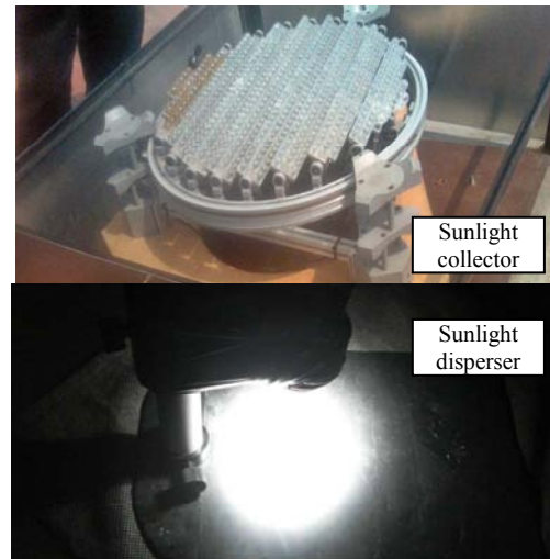
Fig. 2. Photograph of the sunlight collector and dispenser Courtesy: Polymer Optical Fiber Application Center of Georg Simon Ohm University, Nuremberg, Germany
