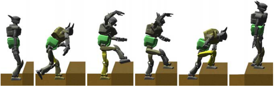
Fig. 4. Stair step planned entirely from scratch
