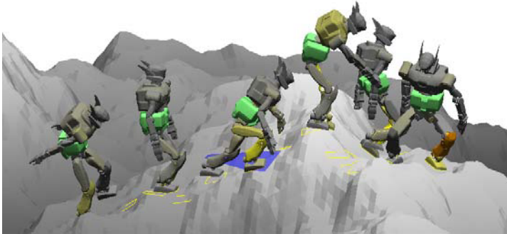
Fig. 12. A motion on steep and uneven terrain generated from a set of several primitives. A hand is being used for support in the third configuration.
