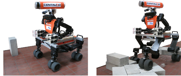
Fig. 1. Our hybrid wheeled-legged mobile manipulation robot Momaro is capable of omnidirectional driving (left) and stepping (right).
