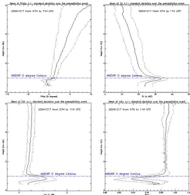
**Figure 2: Mean  $\pm$  standard deviation vertical profiles of  $Z_H$ ,  $Z_{DR}$ ,  $\rho_{HV}$  and  $\Phi_{DP}$  obtained on the 17 December 2004.**
