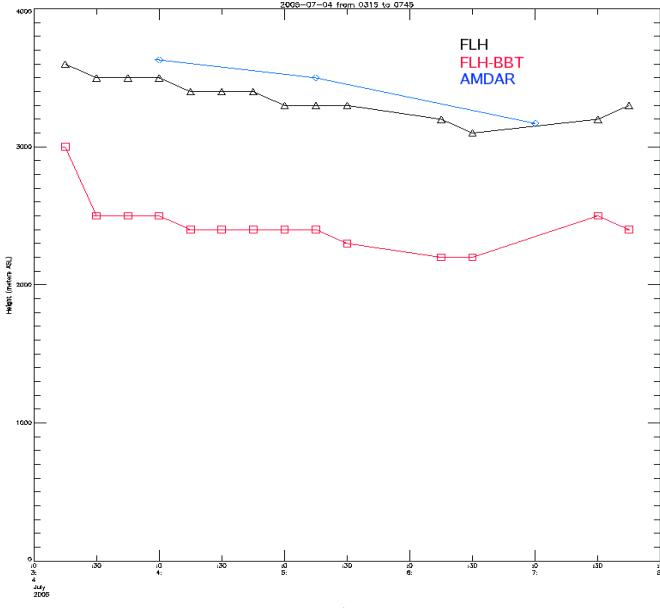
**Figure 6 : a time series of the FLH and FLH-BBT levels retrieved by the method together with AMDAR measurement on the 4 July 2004.**
