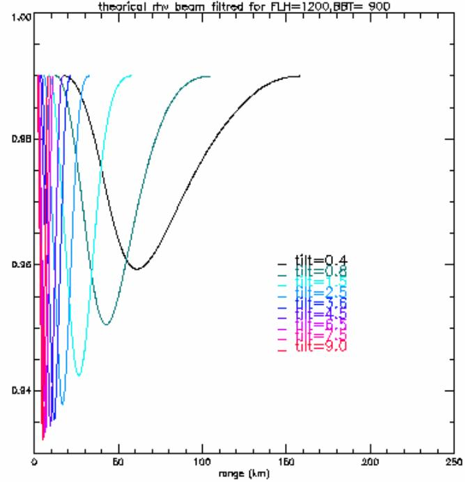
**Figure 5 : An example of a set of simulated curves for FLH=1200 m and BBT=900 m , which is the (FLH,BBT) couple that gives the best fit with the observed  $\rho_{\text{HV}}(r)$  curves presented on Fig. 4.**
