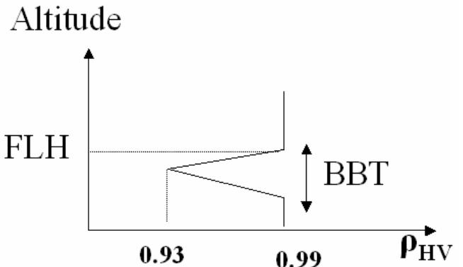
**Figure 3: Proposed conceptual model for the vertical profile of  $\rho_{HV}$ .**
