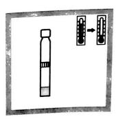
Blank-vial and Samplevial: Allow to cool down to room temperature in a cooling rack.
