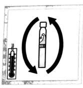
8. Blank-vial and Samplevial: remove the hot vials. Carefully invert twice.
