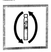
5. Blank-vial and Samplevial: Invert to mix.
