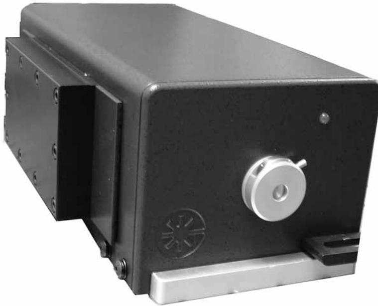
Laser (MTM) head shown with water cooled heatsink. Clamp not included.
