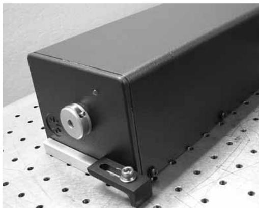
**Figure 3-5. Secure System to Optical Table <sup>a</sup>**
