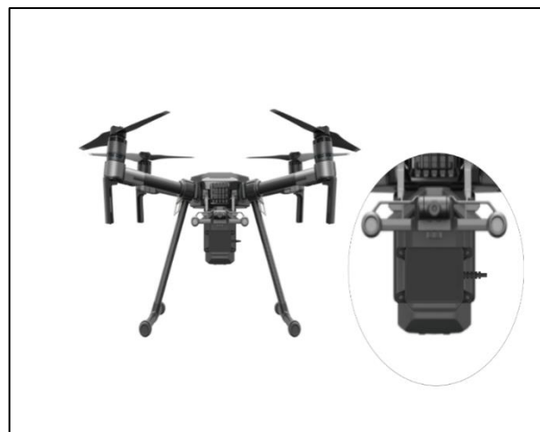
Figure 2 Installation of radar and base
