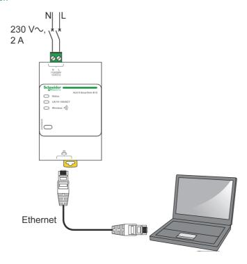
Acti9 Smartlink SI D has an embedded web server. A web server is used to set Ethernet parameters or to display PowerTag energy sensors configured with Ecoreach software, see *Ecoreach Online Help*.
