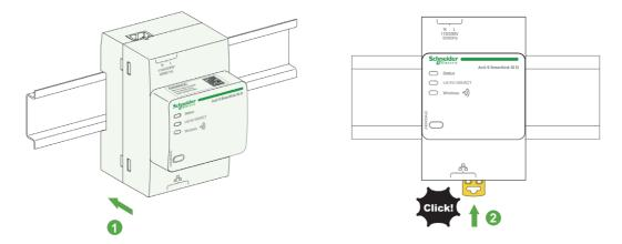
The following table describes the procedure for mounting the Acti9 Smartlink SI D device on a DIN rail:
