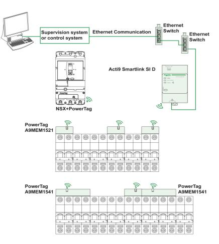
Acti9 Smartlink SI D also manages web pages in order to configure settings or to monitor the wireless devices.
