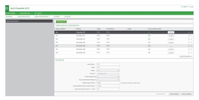
**NOTE:** If you have multiple panels and if each panel has PowerTag energy sensors, then it is recommended to switch on power and commission each Acti9 Smartlink SI D one by one. This helps to discover only the required wireless communication devices specific to each Acti9 Smartlink and avoids discovering the long list of devices.
