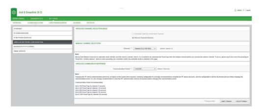
This page allows you to select the wireless channel either automatically or manually. Click **Automatic Selection of the Best Channel** to select the channel automatically.
