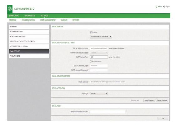
Click the **Enable** check box to configure the email server settings (enabled by default). Acti9 Smartlink SI D allows you to select the **schneider-electric mail server** or **my own SMTP server** profiles from the drop-down list.
