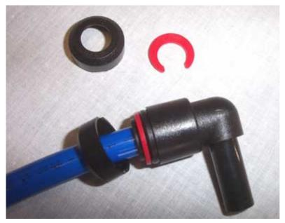
An optional *Locking Clip* (shown red) and *Collet Cover* is available to ensure the fitting will not part in extreme conditions. The clip is essential if the fitting and pipe do not align naturally.
