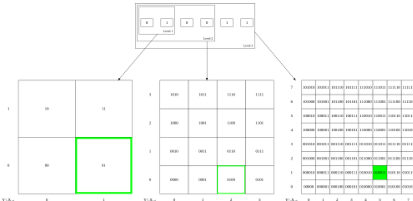
Figure 66. An example for the computation of the Morton index based on the tile coordinates on three levels of a quadtree
