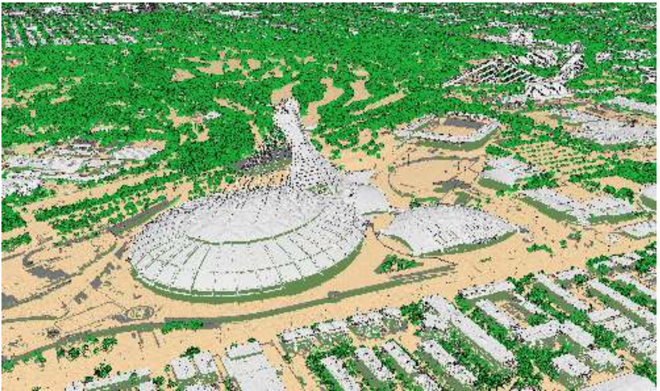
40 billion point cloud from the City of Montreal with ASPRS classification codes (CC-BY 4.0)
