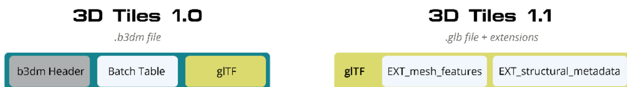
Figure 63. Batched 3D Models in 3D Tiles 1.0, and the corresponding representation in 3D Tiles 1.1
