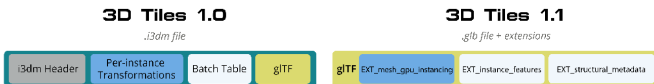
Figure 64. Instanced 3D Models in 3D Tiles 1.0, and the corresponding representation in 3D Tiles 1.1
