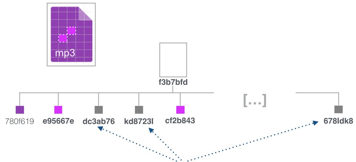
"Unfortunately by dividing a file into fixed size blocks results in all blocks being changed if we to insert a single new byte into the beginning of a file." - Hyperdrive
