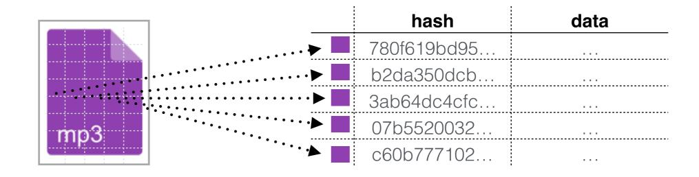
"Unfortunately by dividing a file into fixed size blocks results in all blocks being changed if we to insert a single new byte into the beginning of a file."
