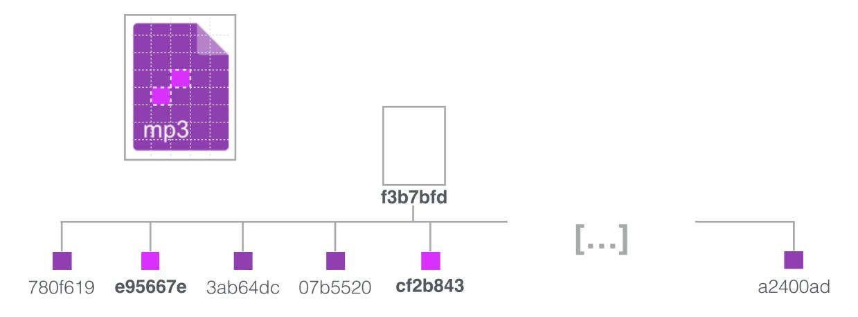
"Rabin fingerprinting is a content-defined chunking strategy that splits a file into varied size blocks based on the file content. [...] Content defined chunking means that **only the neighboring blocks are likely to change** when changing a file." - Hyperdrive Specification
