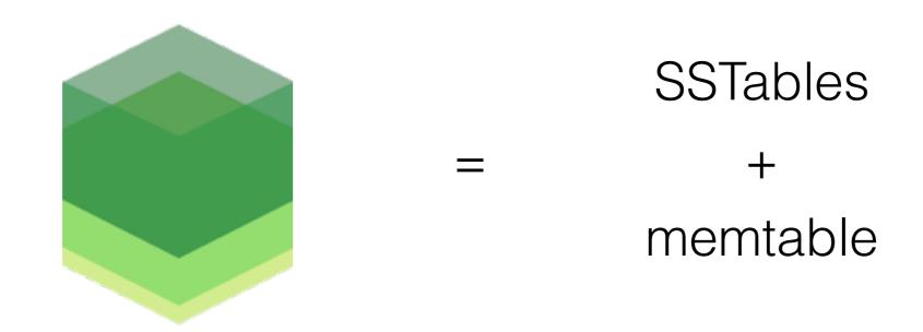
"Take an **SSTable**, add a **MemTable** and apply a set of processing conventions and what you get is a nice database engine for certain type of workloads. In fact, Google's BigTable, Hadoop's HBase, and Cassandra amongst others are all using a variant or a direct copy of this very architecture." - <u>lilya Gregorik</u>
