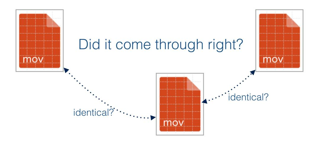
Bit torrent calculates the cryptographic hash for each piece, storing them as a *hash table*
