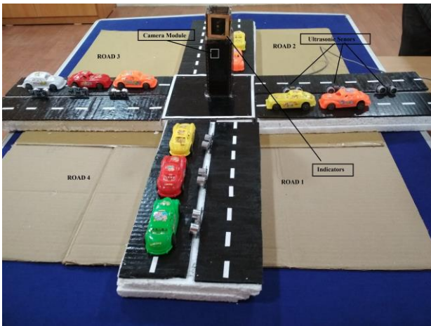
Fig. 5 Four way traffic junction prototype
