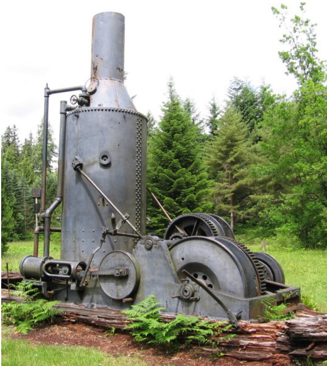
Figure 8: A steam donkey. Source: Rschulz, Wikimedia Commons, GFDL-1.2
