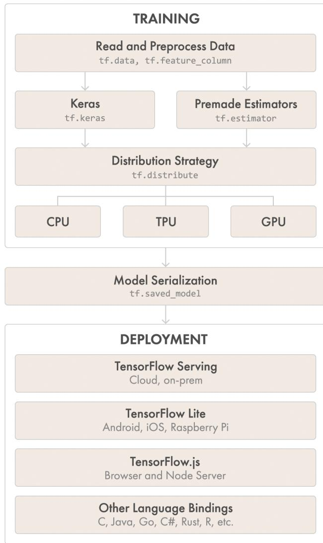
**01** Load the training data using **pipelines** created with `tf.data`. As an input, you can use either in-memory data (NumPy), or a local storage, or a remote persistent storage.
