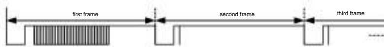
Figure 14-20 The frame format of continuously sending NEC with simple repeat code by pressing the key
