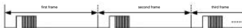
Figure 14-35 Continue to send SONY code frame format continuously by pressing the key
