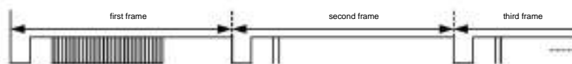
Figure 14-29 The frame format of continuously sending TC9012 codes by continuously pressing the key
