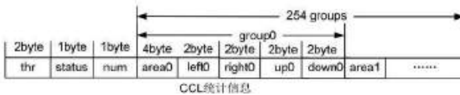
Figure 8-11 Storage of CCL statistics in Memory (sequential storage)
