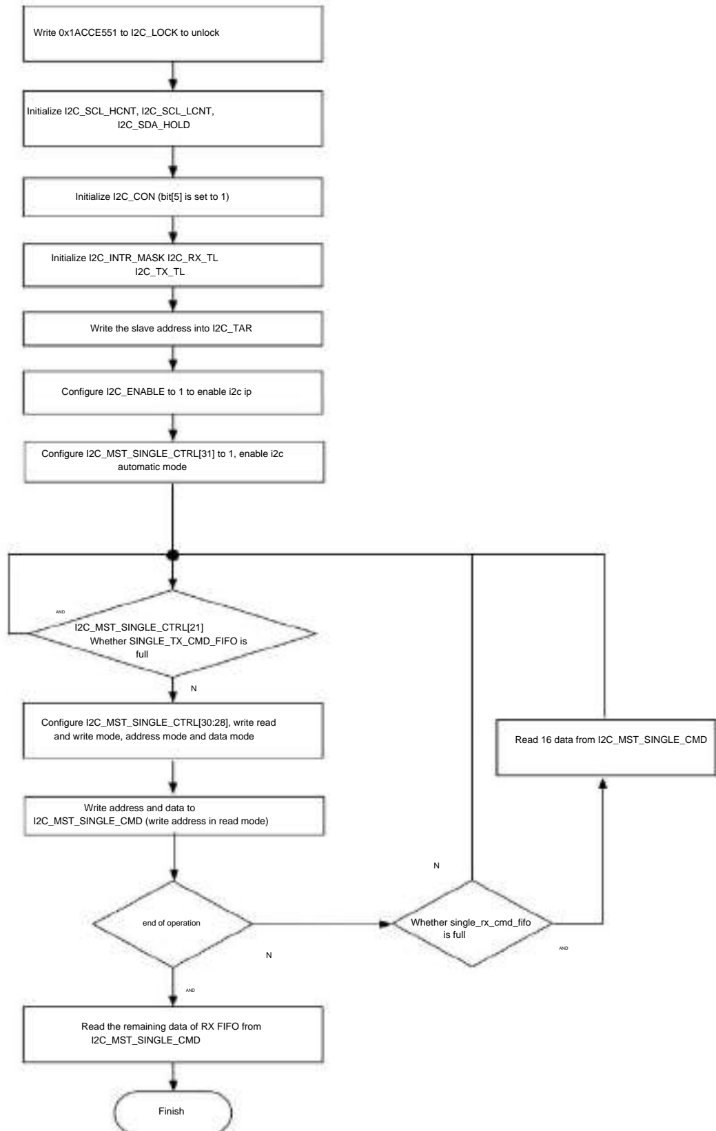
Figure 12-1 Flowchart of sending and receiving data in a single operation of the host
