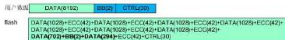
Figure 4-20 Data structure of 8K Page-size in 24bit ECC mode
