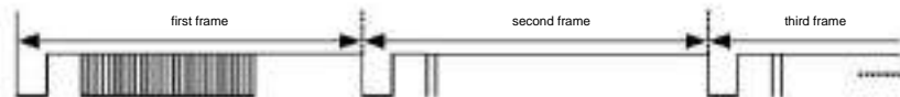
Figure 12-42 The frame format of continuously sending TC9012 codes by continuously pressing the key
