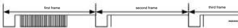
Figure 12-33 The frame format of continuously sending NEC with simple repeat code by pressing the button continuously
