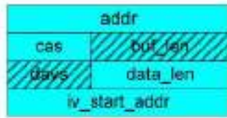
Figure 13-15 Multi-packet encryption and decryption channel link list header structure
