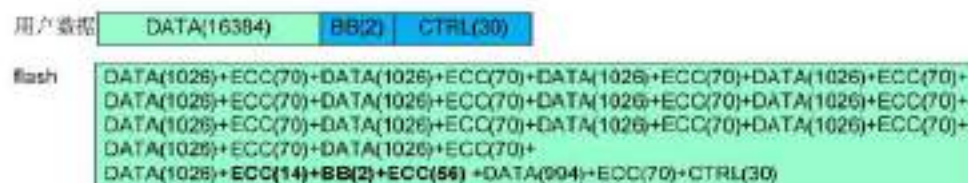
Figure 4-25 Data structure of 16K Page-size in 40bit ECC mode
