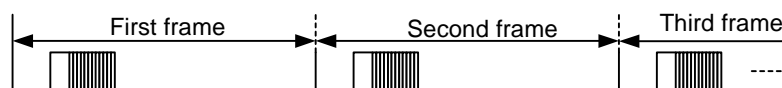
Figure 11-40 Frame format for transmitting continuous SONY codes by holding the key down
