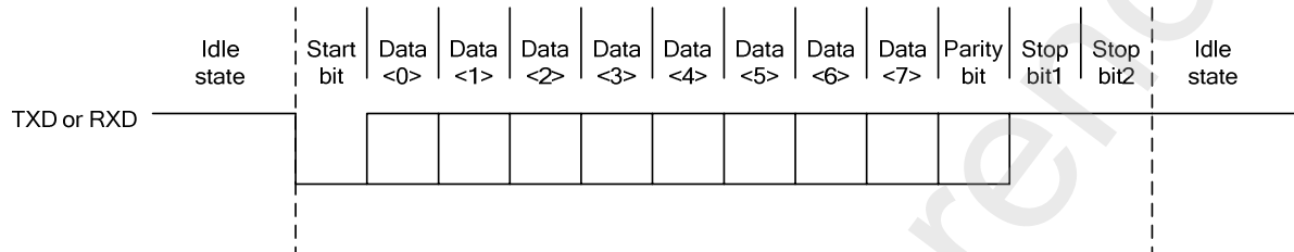
Figure 12-7 Frame format of the UART
