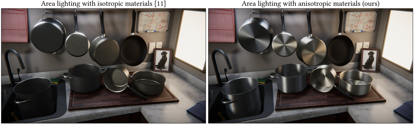
Figure 1: Real-time area lighting with Linearly Transformed Cosines (LTCs) in a commercial game engine. Our LTC approximation for anisotropic materials takes 0.7 ms at 1080p resolution on an NVIDIA GeForce RTX 2080 GPU.
