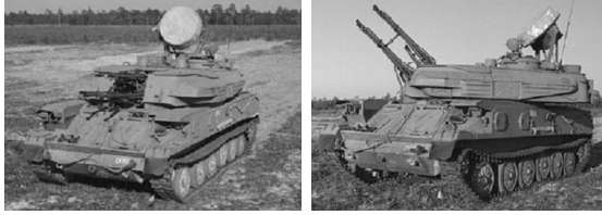
Fig. 22. Target articulation, turret straight and turret articulated of ZSU23/4.
