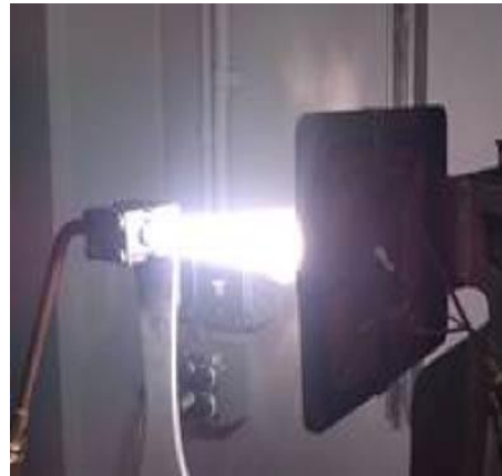
Merlin Nozzle Carbon Coating Development Test
