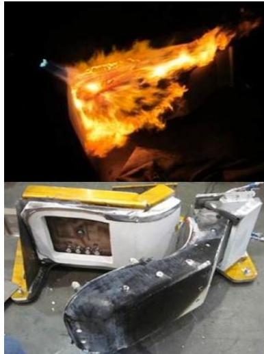
Thermal qualification test of Dragon Claw – connection between Dragon and Trunk
