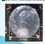
This barium titanate has a large dielectric constant of more than 100,000 at room temperature, which is 30 times greater than that of ordinary barium titanate, and its application in industrial capacitors with a high dielectric constant can be expected. We also discovered that the material has incredible temperature stability, keeping a high dielectric constant in the range from room temperature to 70K (-203.15°C).
