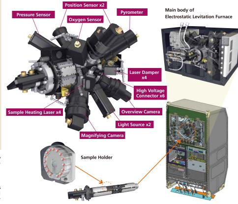
Sample Cartridge **Electrostatic Levitation Furnace** ELF installation image in the
