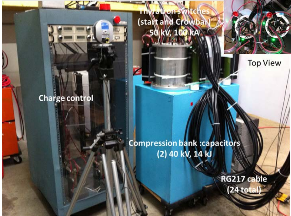
Figure 10. Prototype pulse power system employed on the liner test facility.
