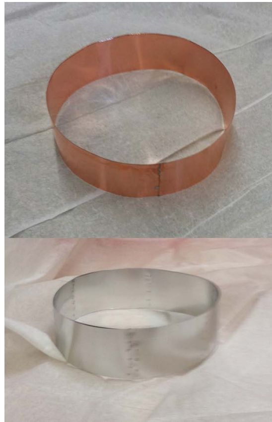
Figure 13. (top) 3 mil copper foil. (bottom) 6 mil aluminum foil
