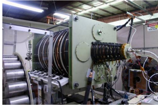
Figure 10. Photograph of the fully assemble ELF, Chamber, and Capacitor Banks
