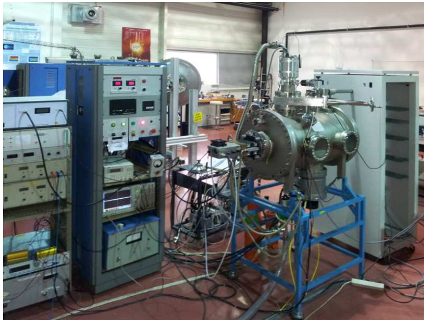
Figure 2.24: Picture of the EPIC test bench with the PEGASES thruster mounted and running.
