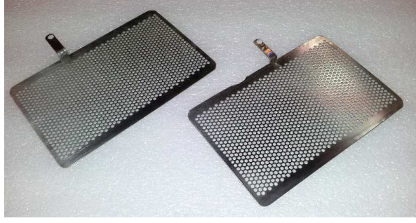
Figure 2.19: The set of grids used for the experiments made out of stainless steel with a transparency of 60 % and a hole diameter of 2 mm
