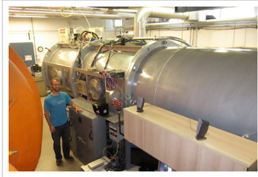
Figure 9 - Vacuum apparatus housing the LiLFA at the EPPDyL.
