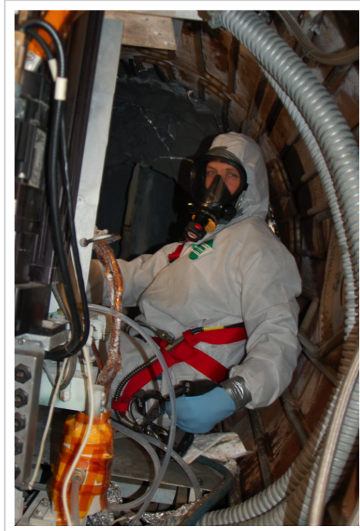
Figure 11 - Cleaning the vacuum chamber after firing the LiLFA.
