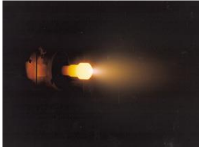
1999 Test Firing of a Primex (now Aerojet) MR-510 Hydrazine Arcjet
