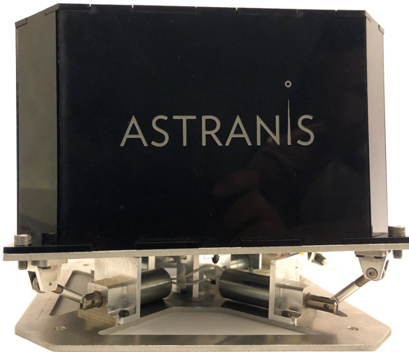
Figure 46. Assembled gimbal with the mock thruster
