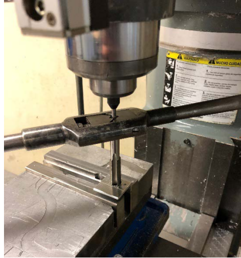
Figure 39. Tapping solenoid threads into solenoid bracket
