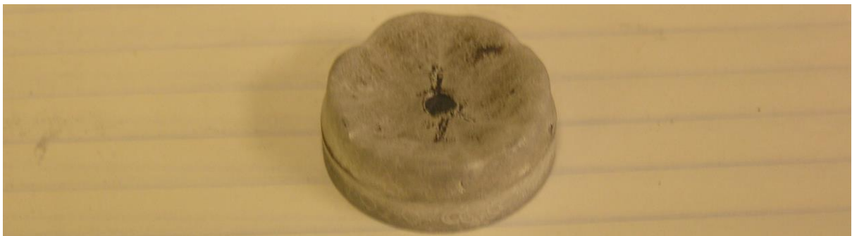
Figure 12.5: Aluminium cathode used in this work
