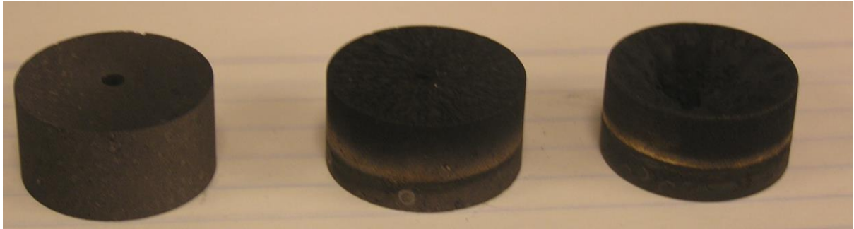
Figure 12.3: Three carbon cathodes; from left to right unused, post bake-out and after significant erosion. Note the colour change from unused to bake-out, indicating compositional change
