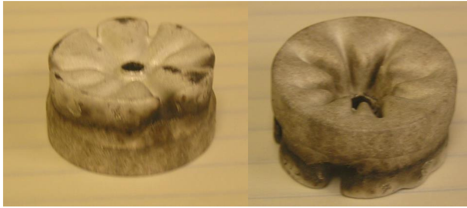
Figure 12.6: Magnesium cathode used in this work, with anomalous erosion trenches shown at left and typical erosion profile at right.
