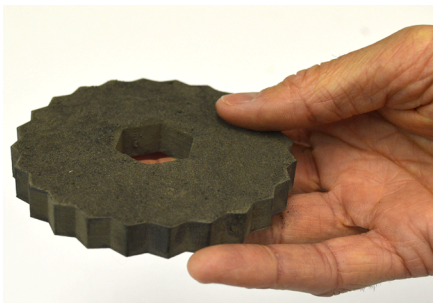
3D printed wrench made by AMF on ISS
