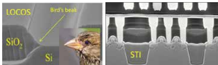
Figure 5-1. Thick-grown isolation oxide or LOCOS (left) and deposited STI used in more recent process technologies (right). The bird's-beak shape concentrates total ionizing dose (TID)-induced hole charge, causing leakage failures at the channel edge. [2]
