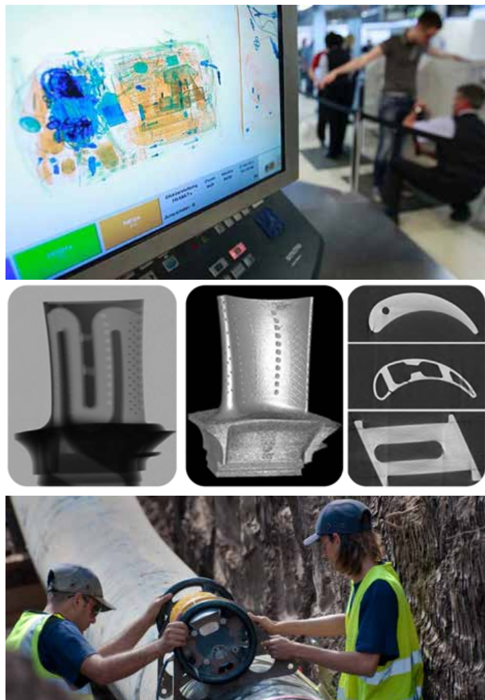
Figure 1-24. X-ray image of the contents of a bag in an airport security line (top); a neutron-produced image of a turbine blade showing interior detail (middle); a portable X-ray machine to scan for pipe defects (bottom).
