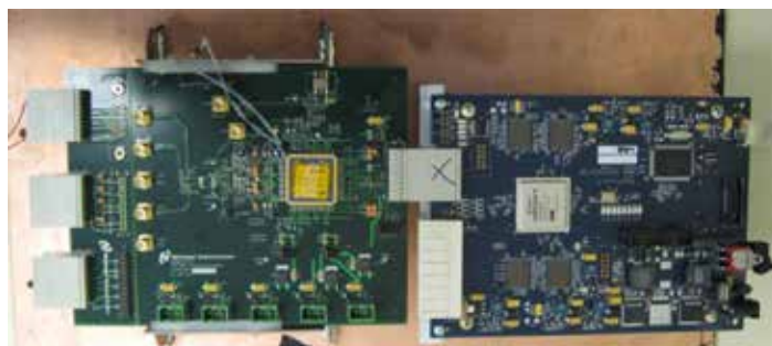
Figure 7-17. A board used for testing the ADC08D1520QML-SP analog-to-digital converter using Texas Instruments' 081000 evaluation board (top). [48] Resistive heaters are attached to the front side of the board to heat the DUT for SEL testing. The DUT is in between the heaters and has been chemically decapped to expose the surface of the die directly to the ion beam.
