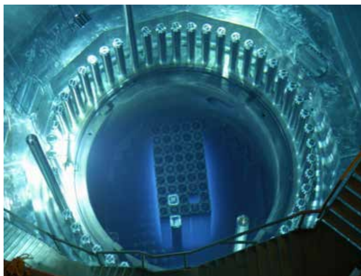
Figure 1-26. Photograph of a nuclear reactor core in operation. The blue color is Cherenkov radiation given off as charged particles pass through the water at speeds greater than the speed of light in water, an effect analogous to the sonic boom produced by aircraft traveling faster than the speed of sound in air.
