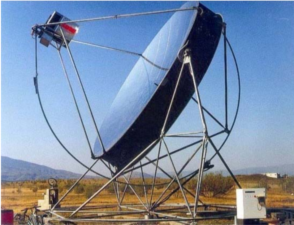
Figure 16: The stretched-membrane parabolic dish concentrator Distal II (Source: PSA, 2004)
