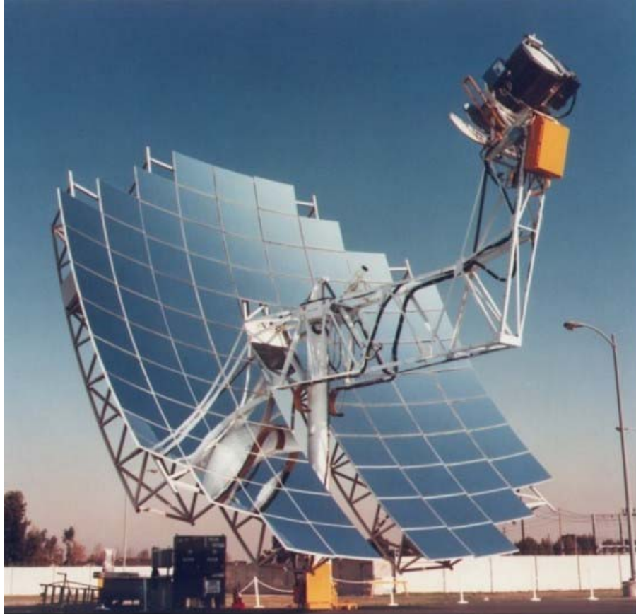
Figure 15: Faceted parabolic dish concentrator with truss support (Courtesy of SES)
