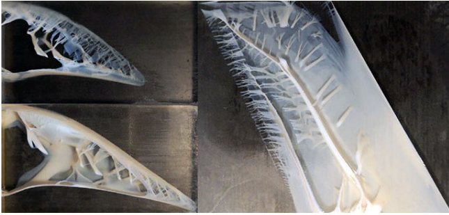
Fig. 16. 3D prints of the slices of the bird beak and the wing structures.
