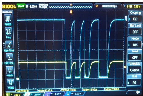
Illustration 1: Signal shape input(yellow) to output(blue) with 1 Node@1Mbps
