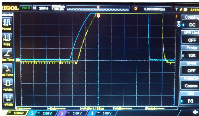
Illustration 3: Signal delay RX(yellow) given a TRX(blue) with 2 Node@1Mbps
