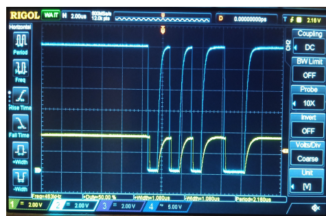
Illustration 2: Signal shape input(yellow) to output(blue) with 2 Nodes@1Mbps
