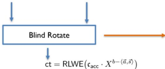
$$\text{Extract}(ct) \rightarrow (\vec{a}_{\text{ext}}, b_{\text{ext}}) + (\vec{a}_{\text{fresh}}, b_{\text{fresh}}) = (\vec{a}_{\text{out}}, b_{\text{out}})$$
