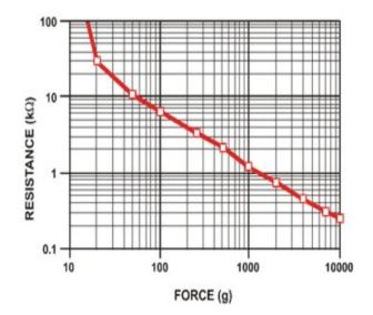
Rreference = 20K Ohms Vout = Vin \* (Rref/Rtotal) Data R: 0x0000~0x3FFF Used FSR range :0.6K ~ 600K Best Resolution at 0.6\*(600/0.6)^1/<sub>2</sub> 20K Ohms
