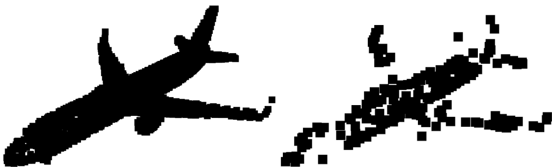
Figure 5.3: Comparison between two airplane point clouds, where all scores greater zero were removed and only scores equal zero stay (left image) and one where all scores equal zero were removed with only scores greater than zero that stay (right image).
