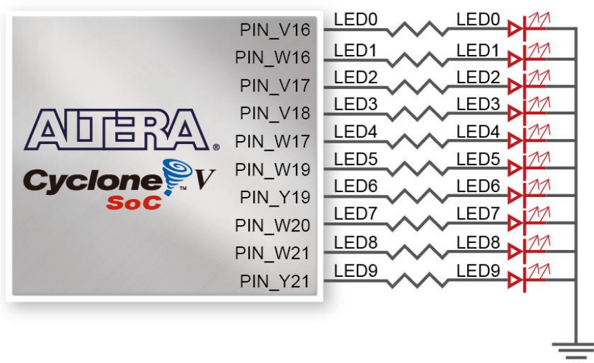
Figure 3-21 Connections between the LEDs and the Cyclone V SoC FPGA
