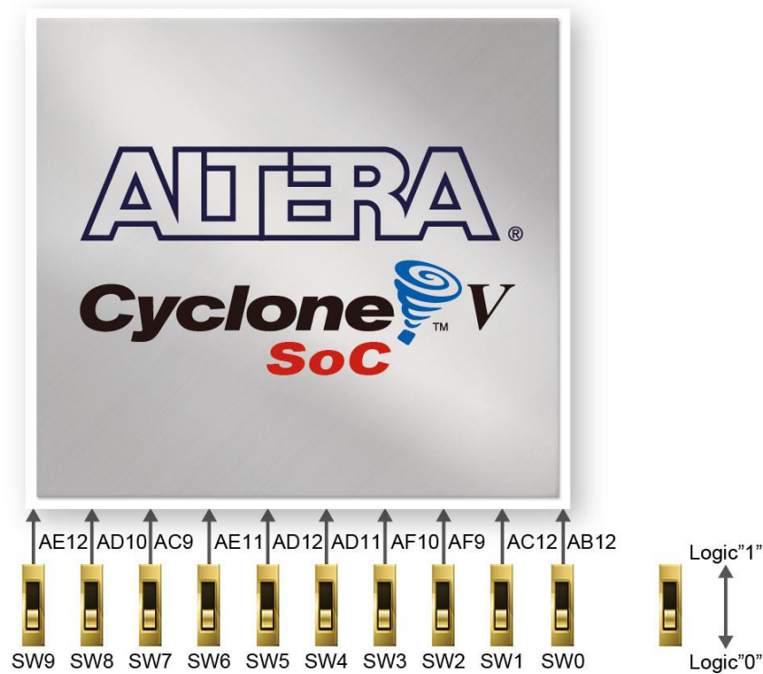
Figure 3-20 Connections between the slide switches and the Cyclone V SoC FPGA
