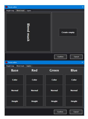
Blend mask defines the way textures are applied to the terrain.
