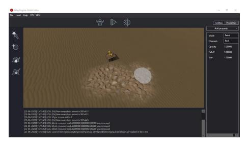
Terrain brush tool allows user to paint the color mask of the terrain.
