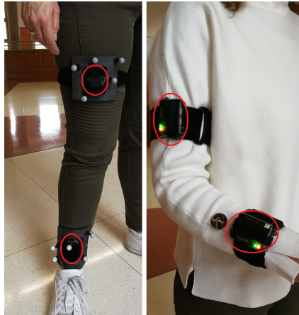
Figure 6.2: IMUs placed at the right lower-limb and at the right upper-limb, marked with red circles. On the left limbs, there are two more IMUs at similar placements than in the right upper-and lower-limbs, respectively. Passive reflector sensors, which are commonly used to obtain optical reference data in biomechanical studies as in [Gar21c], are also shown. However, the optical data are not used in this study.
