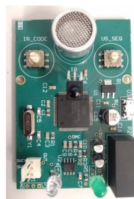
Fig. 3. Aspect of encoded ultrasonic synchronized beacon.
