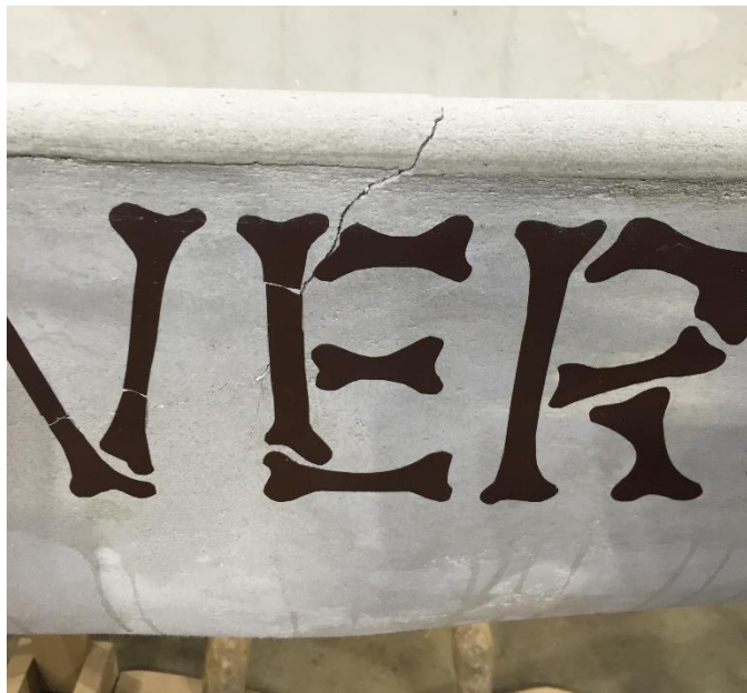
Figure 7: EXTINCTION Structural Crack
