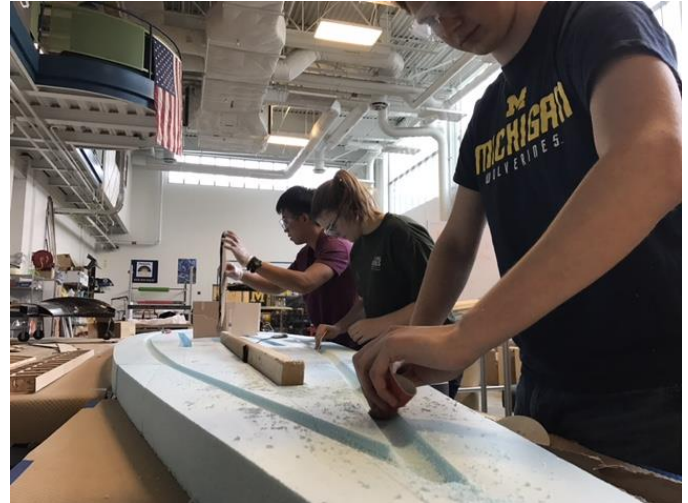
Figure 13: Reinforcement Bars on Mold Base
