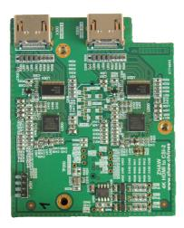
The Institute of Embedded Systems of ZHAW (Zurich University of Applied Sciences) developed a High Definition Multimedia Interface (**HDMI**®) to MIPI®Camera Serial Interface Type 2 (**CSI-2**) converter module (HDMI2CSI) as a plug in to the NVIDIA Jetson TX1 developer kit.
