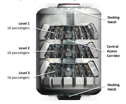
Figure 3. Torpor-Enabled Passenger Habitat Module (48 passengers)
